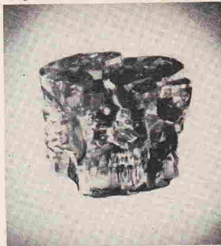
An interesting specimen of Chatham cultured emerald that shows the varied growth pattern developed by the natural heat and pressure method used to grow these man-made gems.
